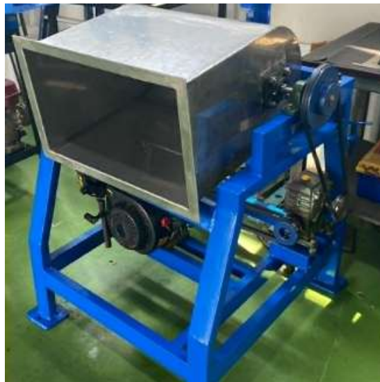
Figure 1 shows the final result of the development of the horizontal bread dough mixer machine in the form of an overall assembly.
